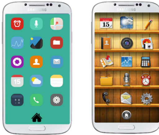
Fig. 2. Exemplary Screenshots of the Smart Phone OS Versions (left side: flat, right side: skeuomorph).
